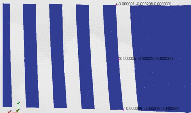
BULGING OF REAR SIDE OF TEETH  $\approx 10 \mu\text{m}$
