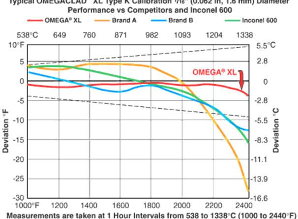
Typical OMEGACLAD" XL Type K Calibration 1/16" (0.062 in, 1.6 mm) Diameter
