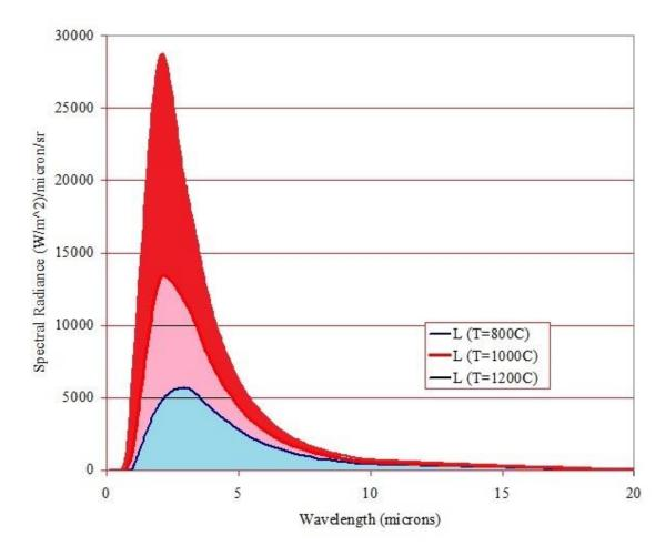
Radiance L(λ,T) can be calculated using Plancks or Wiens law The emissivity and reflectivity sum to 1 for metal surfaces:
