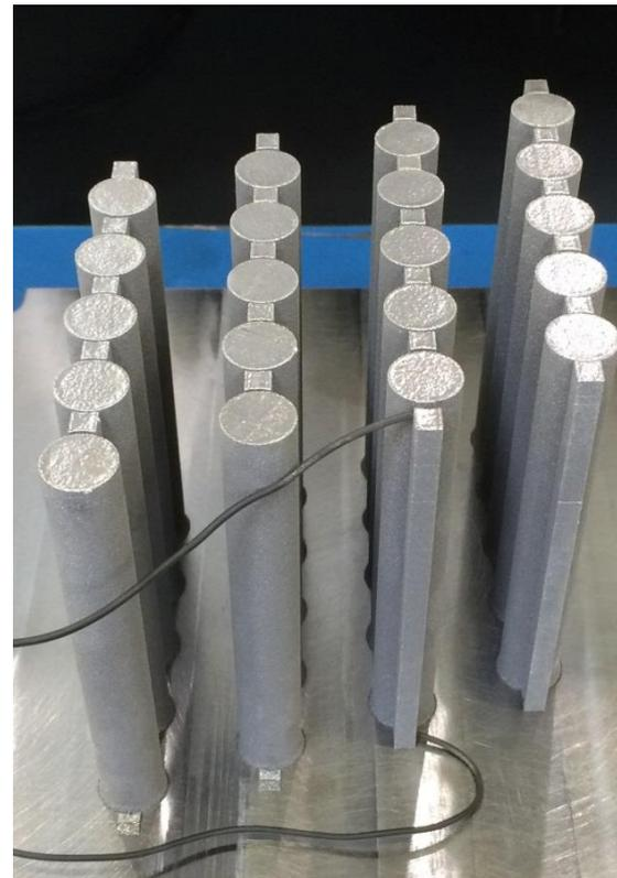
Examples: Titanium parts for tensile strength
