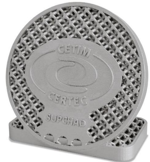
Printed aluminium part, heat treated in model N 250/85 HA (Manufactures CETIM CERTEC on SUPCHAD platform)
