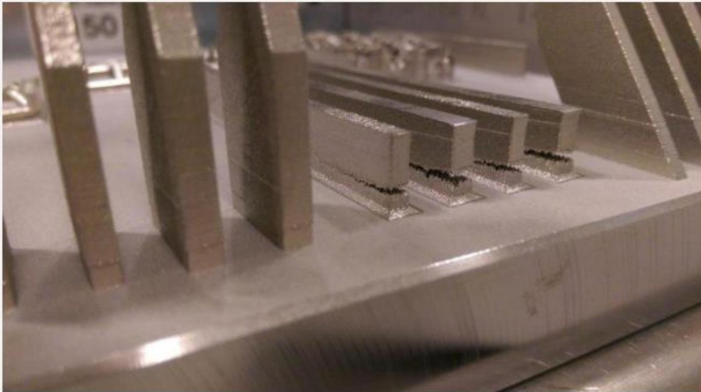
Here, stress buildup shows the collapse of four metal bars created through additive manufacturing. [Photo Credit:
