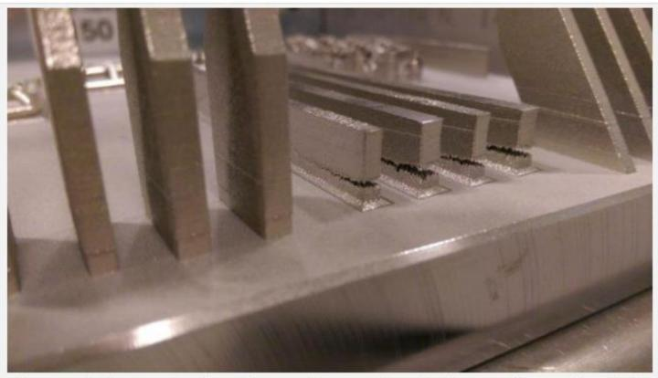
Here, stress buildup shows the collapse of four metal bars created through additive manufacturing. [Photo Credit: Albert To / University of Pittsburgh's Swanson School of Engineering]
