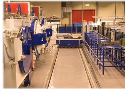
Fully automatic vacuum furnace line Loader 1.500 kg, rotating to both sides
