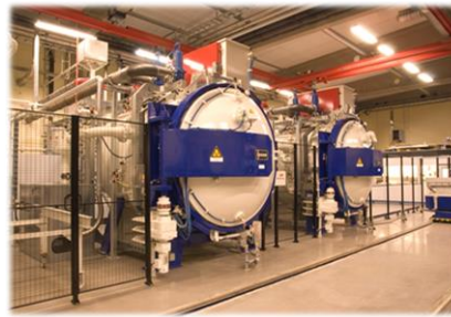
Fully automatic vacuum furnace line Loader 1.500 kg, rotating to both sides
