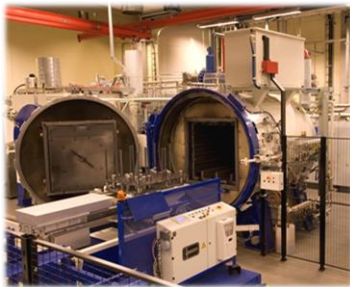
Fully automatic vacuum furnace line Loader 1.500 kg, rotating to both sides
