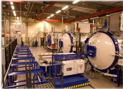
Fully automatic vacuum furnace line Loader 1.500 kg, rotating to both sides
